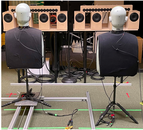
Fig. 1: Photo of the implemented system setup for head translations in the Y direction (front/back).
